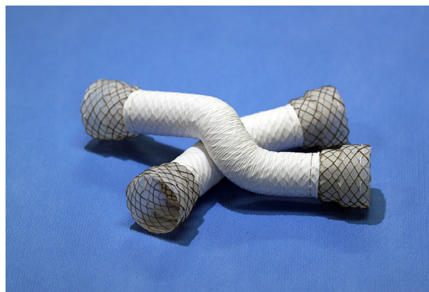
Fig. 1 Photograph of EGIS esophageal stents (S&G Biotech, Seongnam, Korea). The EGIS esophageal stent is knitted from two threads of nitinol wire with a diameter of 0.154 and 0.127 mm, respectively, in a tubular configuration in an interlocking diamond-shaped pattern. The flared ends are coated with silicone, and utilize a unique “double-stepped” shoulders design; the outer shoulders are 24–28 mm in diameter and 13 mm in length, and the inner shoulders are 20–24 mm in diameter and 7 mm in length. The shaft is 16–20 mm in diameter and 4–15 cm in length, and is covered with an ePTFE membrane. The ePTFE membrane is attached to the external surface of the shaft, and is secured with sutures only at its ends. A drawstring made of nylon monofilament is attached to the proximal and distal inner margin of the stent, respectively
